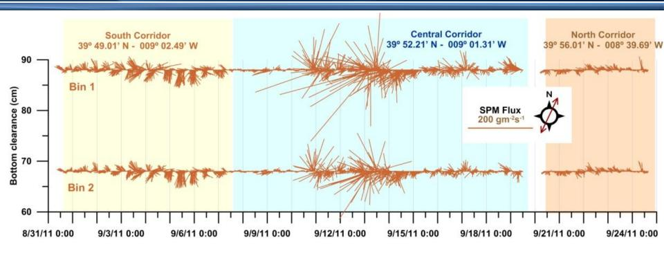
Mass Conc  $_{mg/l}$  x Curr  $_{mm/s}$  x  $\overset{\rightarrow}{Dir}$  = SPM Flux  $_{g/m^2s}$
