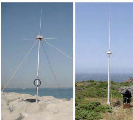
Fig. 2. Old combined Rx/Tx antenna with horizontal whips and new antenna design.
