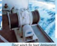
Deck winch for boat deployment (RV MARION DUFRESNE II)
