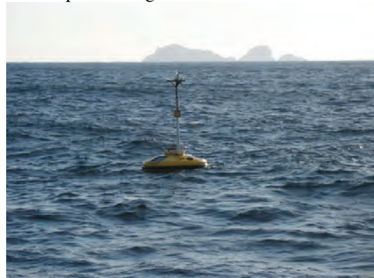
Fig. 4. Deep water MONICAN buoy.
