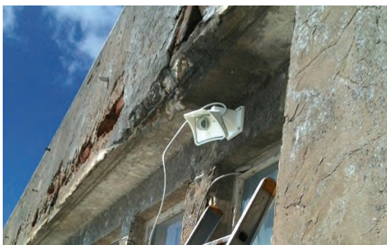
Figure 4. Video monitoring camera located at Sítio da Nazaré. The image viewed by this camera can be observed in the figure 5.
