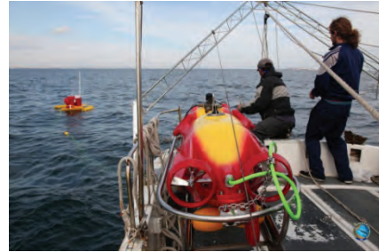
Fig. 4 – AEGIR two-body AUV from Cartagena University
