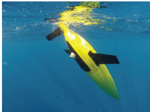
Fig.4. Underwater glider as example of Lagrangian autonomous platform.
