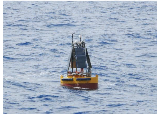
Fig.3. Moored buoy located in Canary Island as example of Eulerian autonomous platform.
