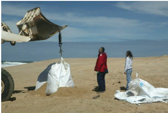
Fig. 3. Native sand collection and weighting during the winter on a spot near the predicted injection point
