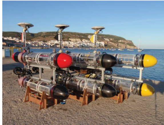
Fig. 2 The MEDUSA-class of autonomous marine vehicles (surface and underwater) – ISR/IST
