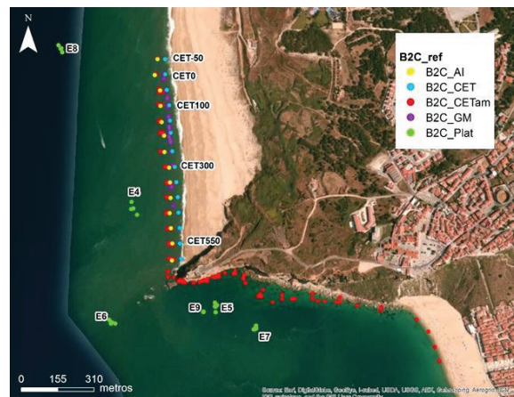
Fig. 5. Tracer experiment plan: B2C_AI – Sediment image analysis; B2C_CET(-50 to 600m) – reference stakes in top of the second beach berm; B2C_CETam - sediment samples of the breaker/swash zone collected each 10 minutes; CET 0 – injection point; B2C_GM – Spotted residual gravel marked located on the top of the swash zone; B2C_Plac – inner shelf samples.
