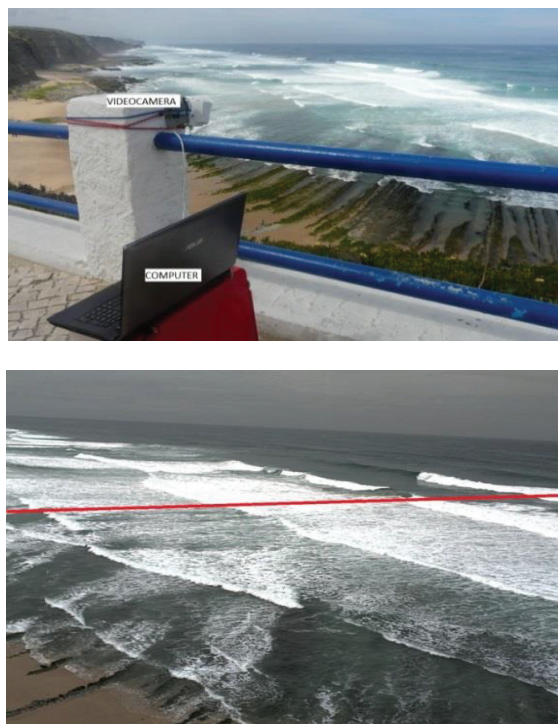
Fig. 2. Video system deployed (above) and an example of a snapshot acquired by the camera (below). Red line indicates the cross-shore transect considered for timestack production and wave celerity computation.
