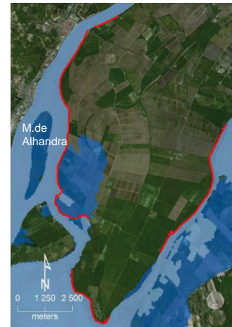
Fig. 3. February 2010 flooding event in LGVFX: reconstruction of the flood affected area (red line); model results for the 2010 event (light blue) with SLR (dark blue) (image: ESRI Aerial Imagery).
