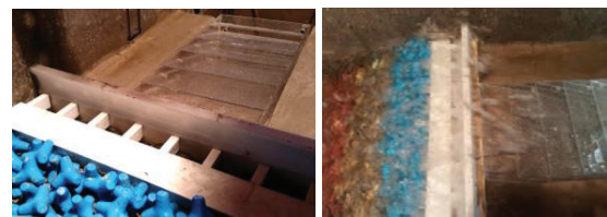
Fig. 5. Sketch of the equipment (with 6 overtopping trays) used for measuring travel distance of mean overtopping discharges. View of the equipment and of an overtopping event during a physical model test.
