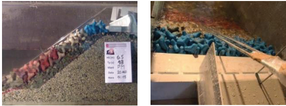
Fig. 3. Left: physical model, side view through the window of the wave flume. Right: top view of the model and of the wave gauge placed over the breakwater armour.
