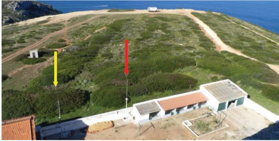
Fig. 1. Photo of Espichel Station, taken from the top of the lighthouse. SeaSonde antenna marked in red and buoy communications antenna marked in yellow.
