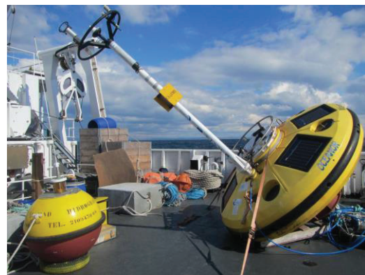
Fig. 3. Oceanographic Datawell Waverider (left) and Meteo-oceanographic Oceanor Wavescan (right) buoys (image © Instituto Hidrográfico).
