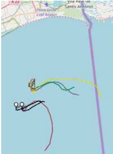
Fig. 1. Buoy and model trajectories. Buoys: black lines; Model runs: line colours as in Table II.
