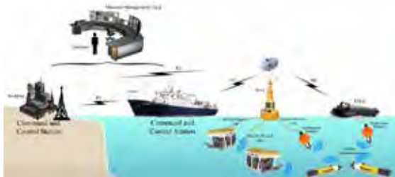
Fig. 1. The main components of a SWARMS scenario. Command and Control Station can be allocated on shore or on ship.
