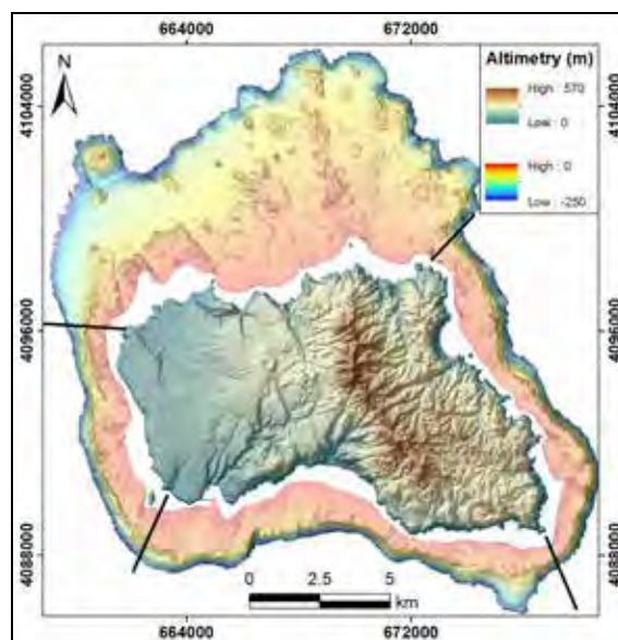
Fig. 3. High-resolution bathymetry of Santa Maria island shelf. Black lines delimit the shelf sectors considered in this study. Map in projection UTM 26S.
