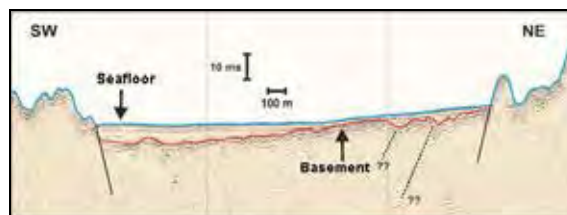
Fig. 7. Boomer seismic profile showing the structural control of the thickest sediment depocenters. Location of profile in Fig. 6.
